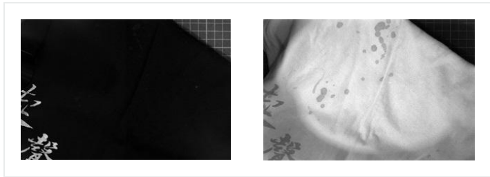
Black t-shirt stained with blood; left room light and no camera filter, right 415nm illumination and Longpass IR 715nm camera filter.
